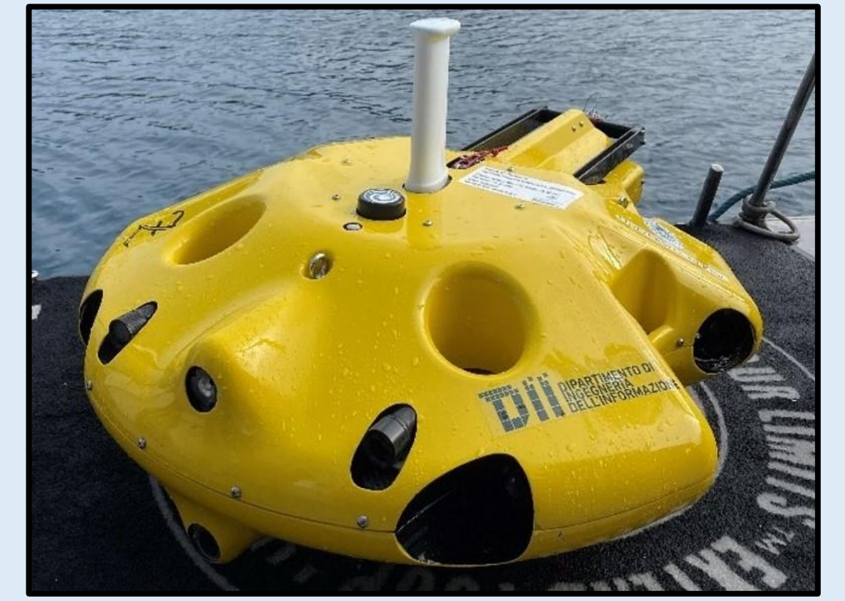
Fig. 2: Zeno AUV – Reference underwater vehicle utilised during the tests
